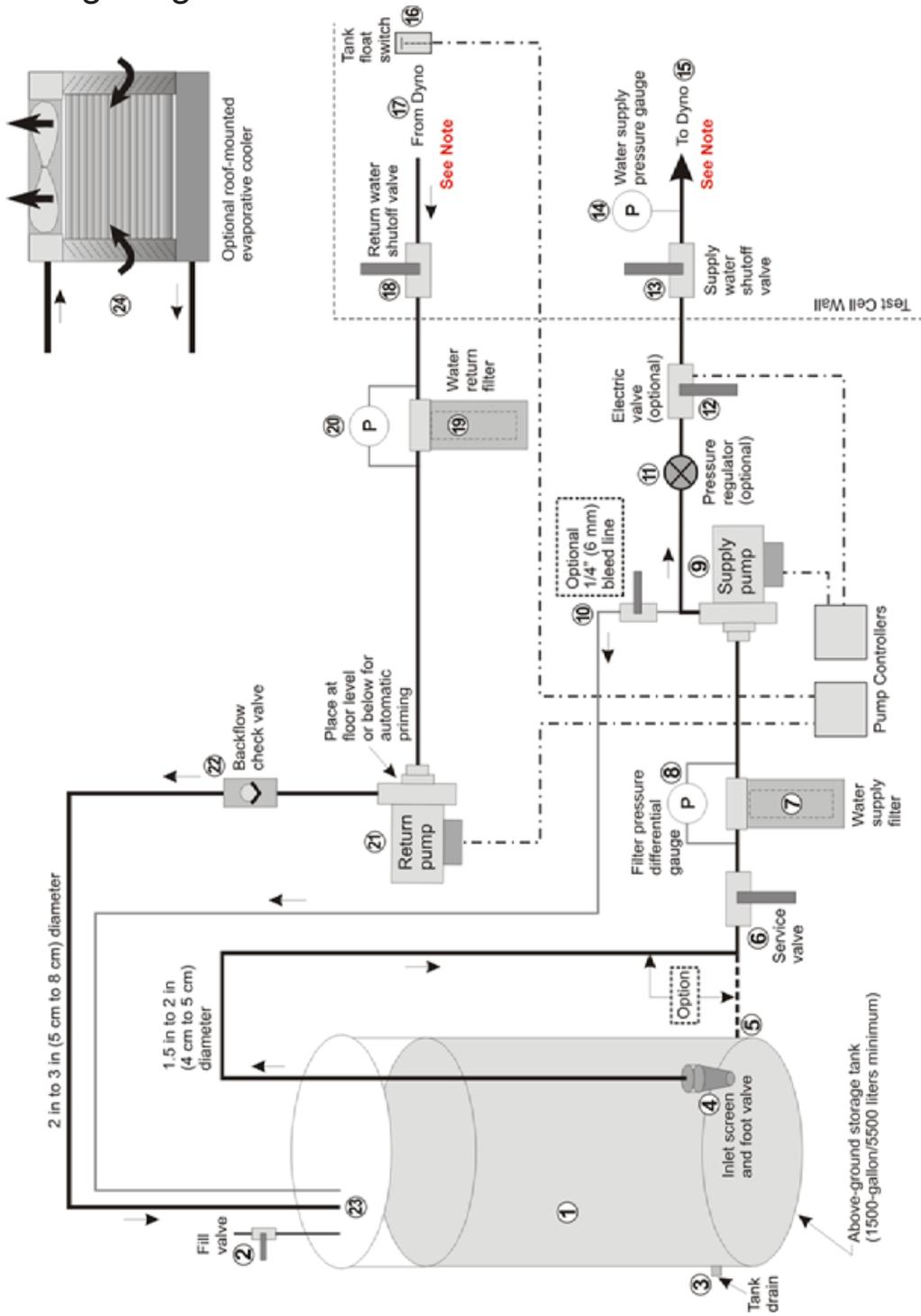
**NOTE:** The water line to the dyno inlet is routed to the left side of the dynamometer as looking at it from the back of the test cell. The water line from the dynamometer is routed to the right side.
