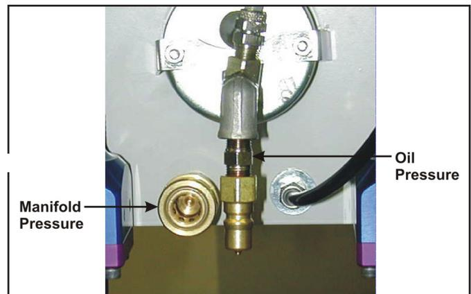
Figure 4.5 Absorber Stand Gauge Connections
