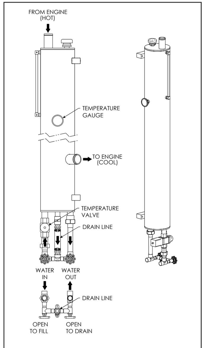
Figure 4.6 CT700-NOP Unpressurized Cooling Tower
