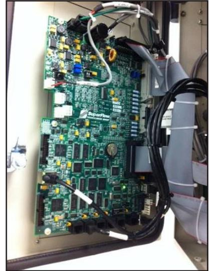
2. In the upper right hand corner located under the gray ribbon cable you will find two blue potentiometers.
