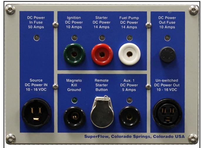
Figure 3.8: Engine Control Panel
