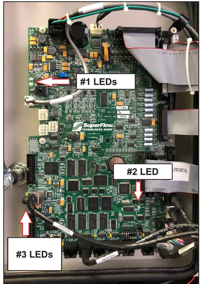
Figure 6.1 2640 Circuit Board LEDs
