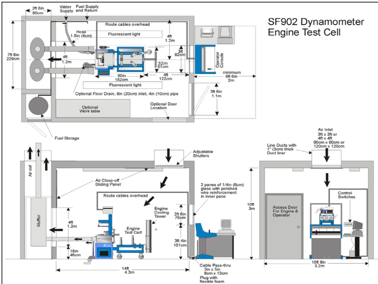
Figure 4.1: Recommended Test Cell Layout
