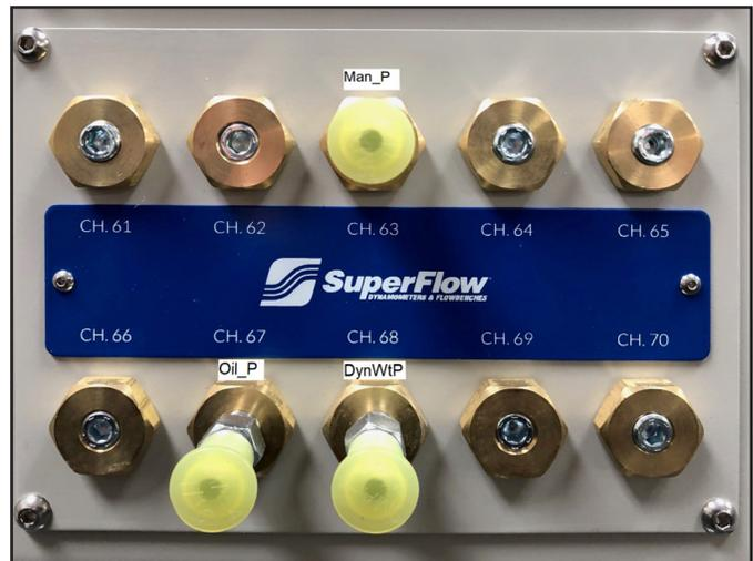
Figure 3.7: Pressure Input Panel
