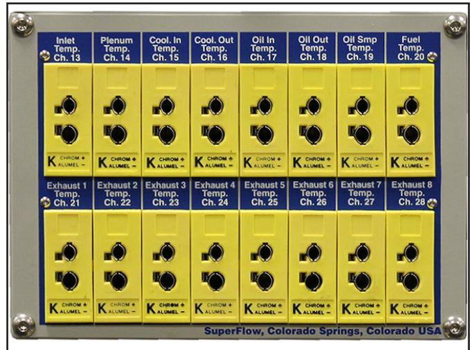
Figure 3.6: Thermocouple Input Panel
