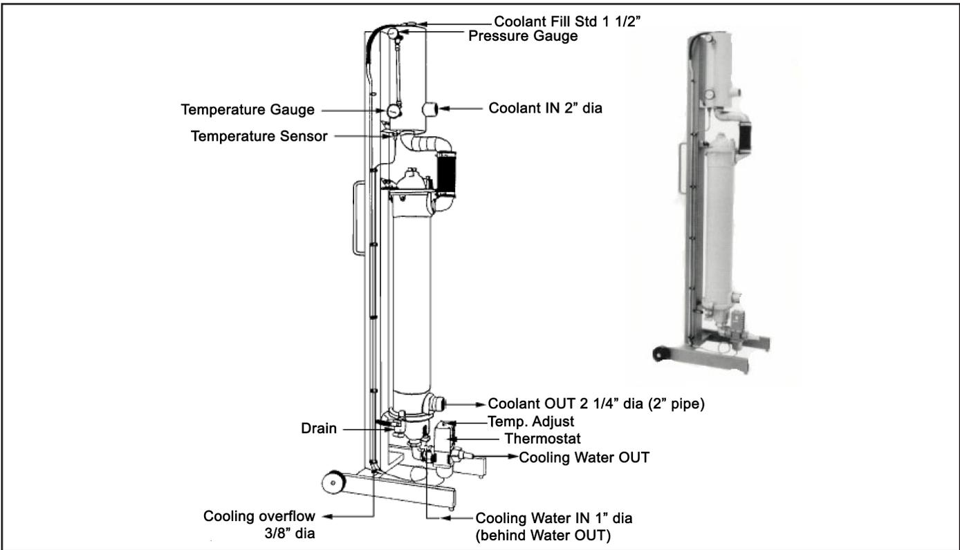
Figure 4.6 CT700P Pressurized Cooling Tower
