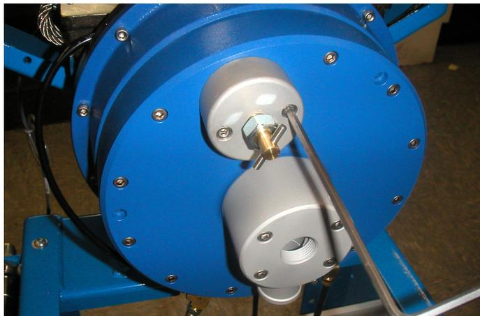
5. Fashion a cork or rubber stopper to fit tightly into the seat of the stator housing. The cork or stopper must be trimmed so that it does not protrude out of the seat more than 1/8".
