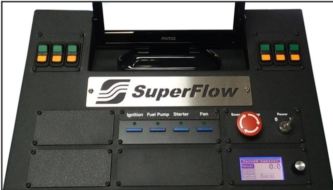
Figure 5.7: Operator Console Controls
