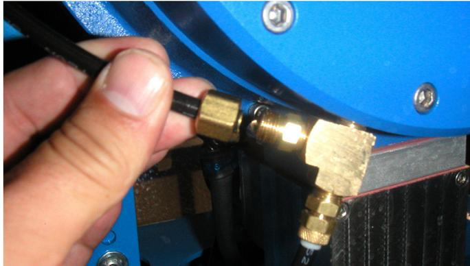
8. Re-install the capacity valve with the valve still in the fully open position.
