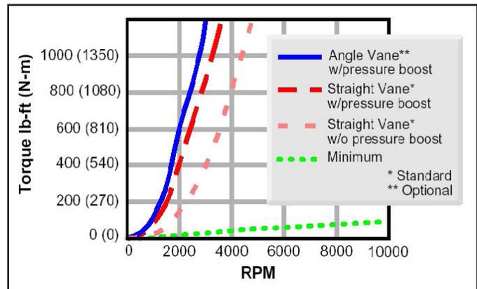
Figure 3.3: SF Water Brake Absorber Torque Capacity
