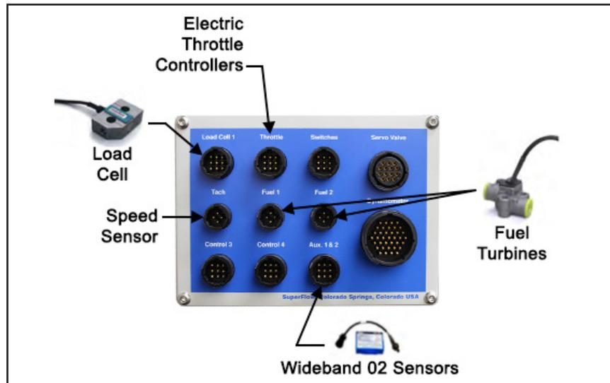
Figure 4.10 Sensor Interconnect Panel
