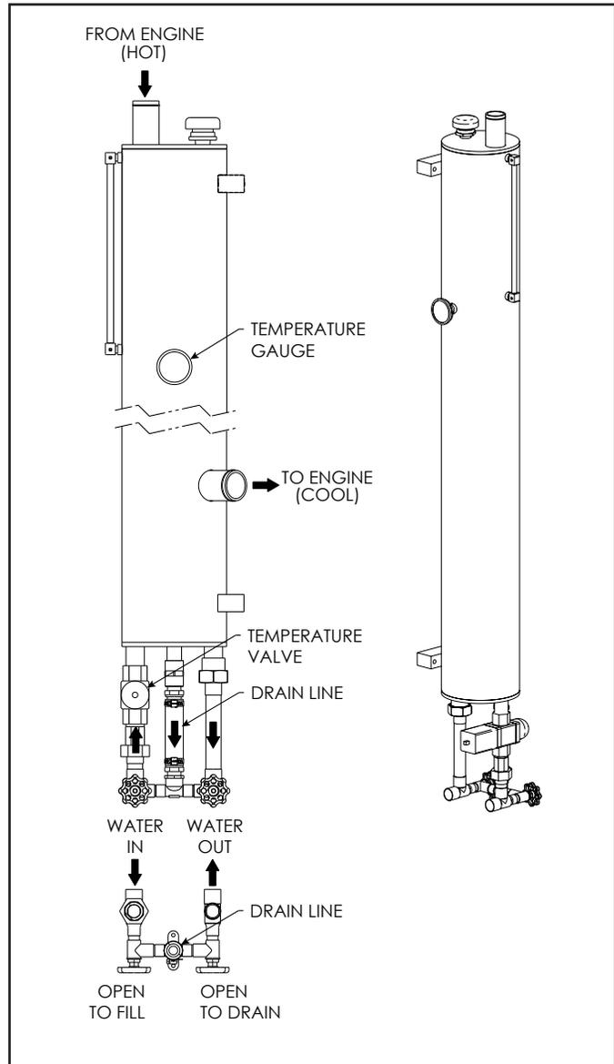
Figure 5.4 CT700-NOP Unpressurized Cooling Tower
