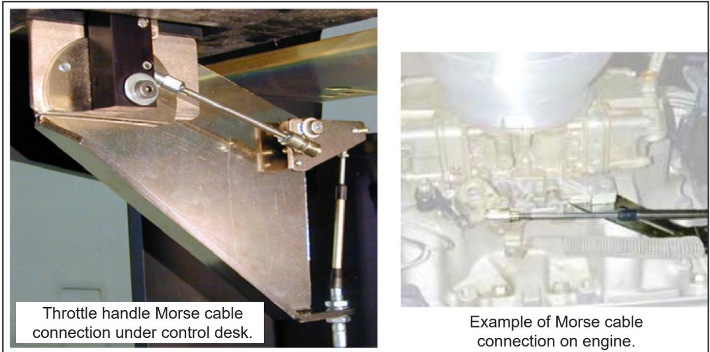
Figure 5.5 Morse Cable Throttle System
