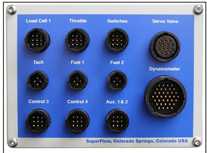
Figure 3.5: Sensor Interconnect Panel
