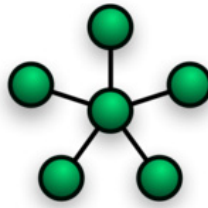
Figure 8-1. Star Network Layout
