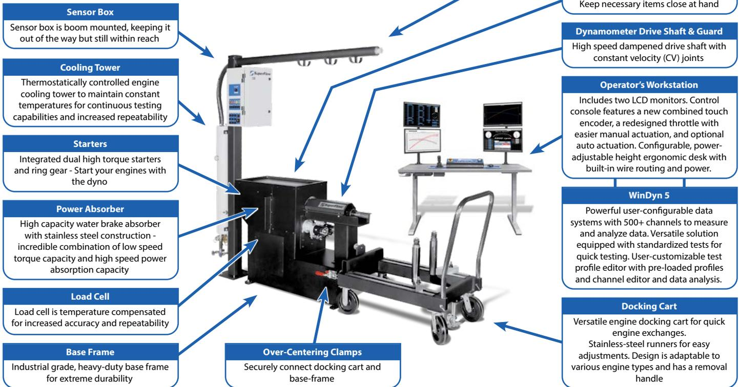
The SF-3000BW (Black Widow) is built with integrated starters which eliminate the need for bell housing or engine mounted starter. A special compliant driveshaft that absorbs the torsional vibrations of the engine allows for coupling to the dynamometer directly to the engine's crankshaft or flywheel. The driveshaft's 4.5 in (114 mm) constant velocity (CV) joints ensure smooth power transfer.
