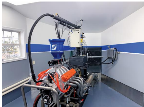
To obtain repeatable test results, begin every "pull" at the same engine temperature.
